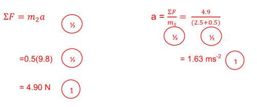
(b) Calculate the magnitude of the tension in the thread.
